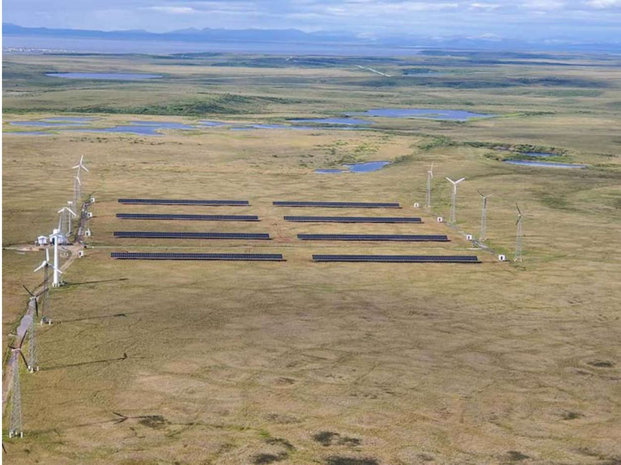
Figure 3. Kotzebue’s wind turbines and solar PV arrays, which use the old wind turbine’s inverters. Image from Misbrener (2021)
