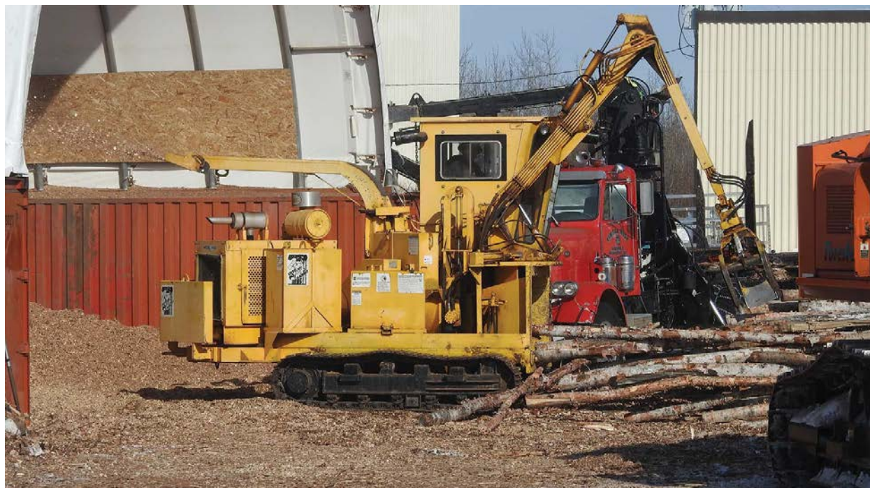
Figure 2. SEGA’s self-propelled chipper and self-loading log truck harvesting wood for the biomass boiler. Image from Orr (undated)
