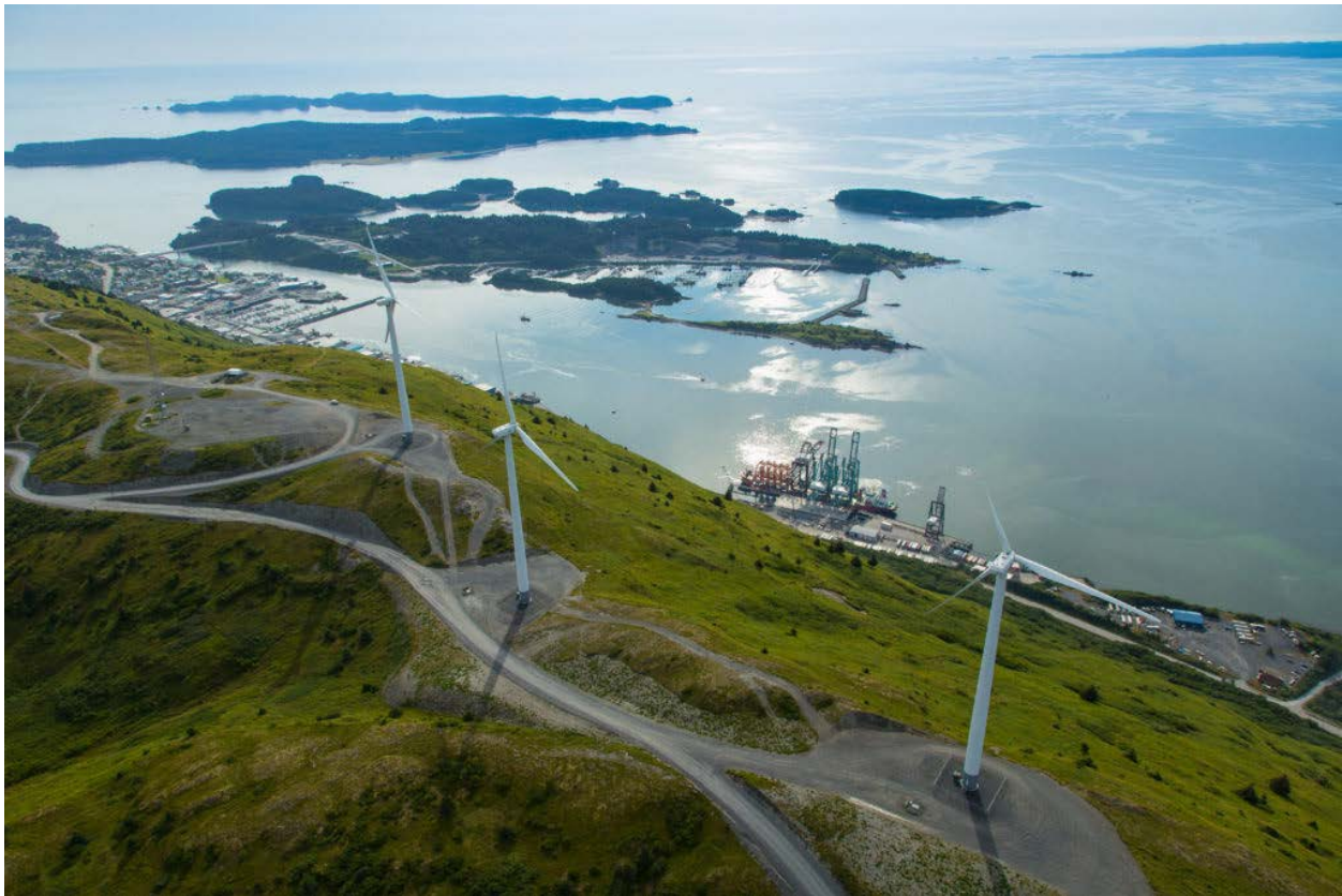
Figure 5. Three GE 1.5-MW wind turbines in Kodiak’s Pillar wind energy project overlook the flywheel-powered electric shipping crane. Image from Kodiak Electric Association (undated)
