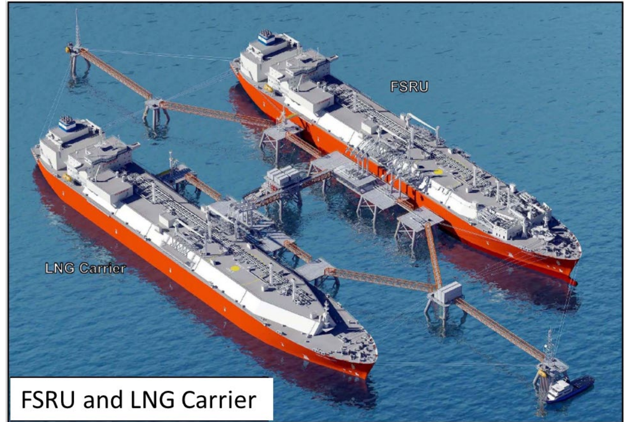
FSRU size in the image: LNG storage capacity of 150,900 m 3 (appx.3.4 Bcf); length of 291 m and a design draft of 11m
